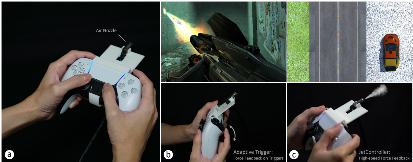
Figure 1: (a) JetController design for the Sony DualSense controller consists of one backward air nozzle, (b) provides recoil feedback by Adaptive Trigger, and (c) generating high-speed force feedback by JetController to support the tactile (surface texture) feedback in racing games. (note: the white smoke is only shown for illustrative purposes, and compressed air jets are invisible in actual use.)
