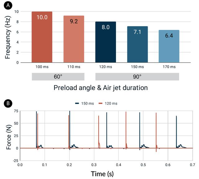
Figure 8: Impact: a) measured impact frequencies across air jet actuation durations at  $60^\circ$  and  $90^\circ$  preload angles; b) example measured force response curves for the  $90^\circ$  preload angle at  $8.0Hz$  and  $7.1Hz$ .
