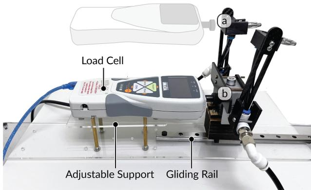
**Figure 5: Experimental setup for force measurement using a load cell at two impact locations.**
