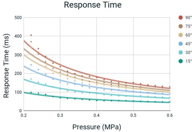
Figure 7: Response time across preloaded angles and air pressures.
