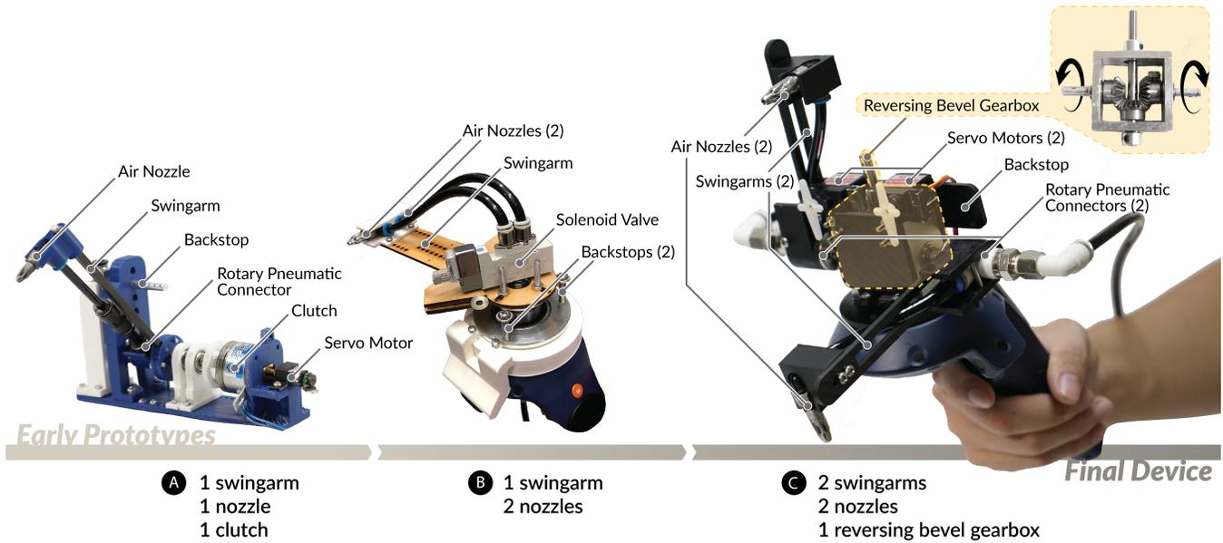
**Figure 3: System design evolution: a) Single-swingarm + single-nozzle design that rewinds to initial position using a servo motor and electromagnetic clutch; b) Single-swingarm + two-nozzle design that eliminates rewind time, but causes significant shift in balance; and c) Final *reciprocating dual-swingarm design* with a reversing bevel gearbox to eliminate gyro effects, to minimize shift in balance, and to achieve high-frequency impact force feedback of 10Hz.**
