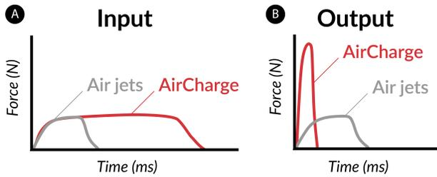
**Figure 2: Impulse is the force applied over time, or the area under a force-time curve: a) AirCharge extends the input force duration to accumulate momentum, i.e. increased area under the force-time curve; b) AirCharge shortens the output force duration, resulting in an output force-time curve with increased force magnitude.**
